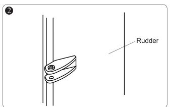
▶ Please note that Epoxy glue must be apply to these holes before screw the control horn to the rudder. If not, it comes off during flights, you may lose control of your airplane, resulting in an accident!
