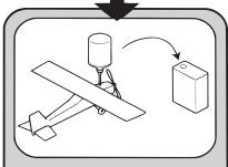
Empty the fuel tank after flying, fuel left in the tank can cause corrosion and lead to engine problems.
