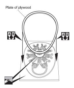
5. Using a 3mm drill bit, enlarge the four holes in the cowling.
