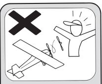
**ALWAYS** adjust the engine from behind the propeller, and do not allow any part of your body to be in line with the propeller.
