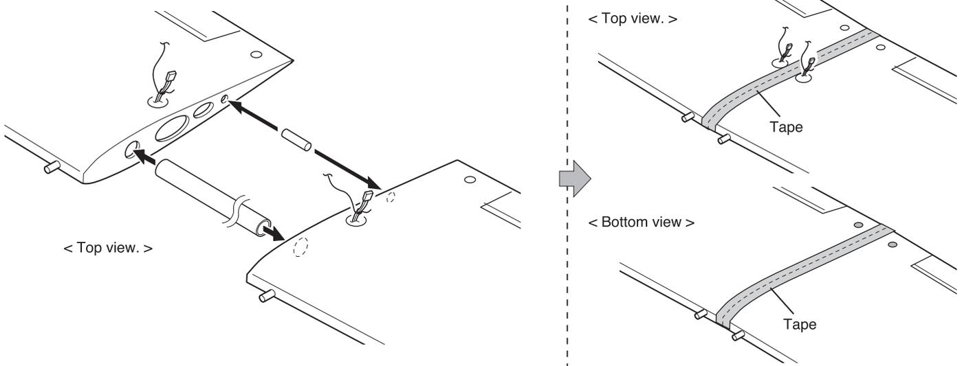
**INSTALLING THE MAIN LANDING GEAR**
