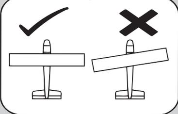
Check that the wings are correctly fitted to the fuselage.
