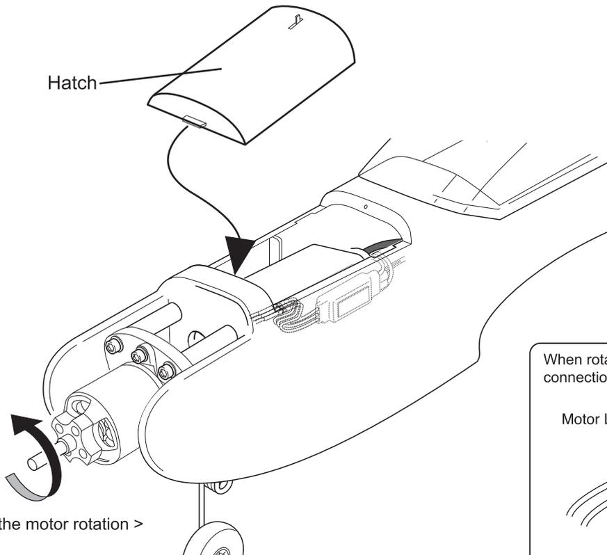
When rotating clock wise, change the connection of 2 wires.
