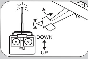
Operate the control sticks on the transmitter and check that the control surfaces move freely and in the **CORRECT** directions.
