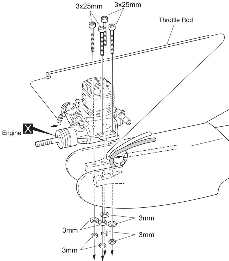
Engine Mount is adjustable for various size of engines. Before mounting engine, loosen 4mm screws and adjust engine mount size before installing engine.
