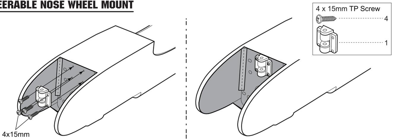
**INSTALLING THE NOSE GEAR**
