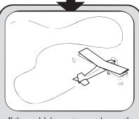
If the model does not respond correctly to the controls, land it as soon as possible and correct the fault.
