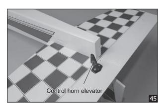
7. Attach clevis to the third hole in the control horn.
