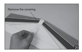
6. When you are sure that everything is aligned correctly, mix up a generous amount of 30 minute epoxy. Apply a thin layer to the top and bottom of the stabilizer mounting area and to the stabilizer mounting platform sides in the fuselage. Slide the stabilizer in place and re-align. Double check all of your measurements one more time before the epoxy cures. Remove any excess epoxy using a paper towel and rubbing alcohol and hold the stabilizer in place with T-pins or masking tape.
