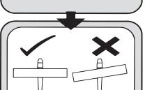
Check that the wings are correctly fitted to the fuselage.
