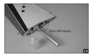
7) Mix a generous amount of 30 minute epoxy. Coat the exposed half of the dihedral brace, the wing joiner box and both root ribs with epoxy. Slide the two wing halves together and carefully align them at the leading and trailing edges. Wipe away any excess epoxy using paper towels. Use masking tape wrapped around the center section to hold the halves in place until the epoxy cures.
