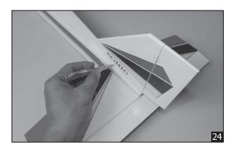
Now, remove the vertical stabilizer and using a modeling knife, carefully cut just inside the marked lines and remove the film on both sides of the vertical stabilizer. Just as you did with the horizontal stabilizer, make sure you only press hard enough to cut the film, not the balsa vertical stabilizer.
