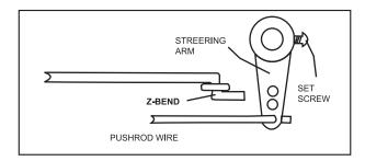
7. Locate the nose gear wire. Slide the nose gear wire up through the lower portion of the nose gear block, then through the nylon steering arm, then through the upper portion of the nose gear block. The top of the nose gear wire should be flush with the top of the nose gear bracket.
