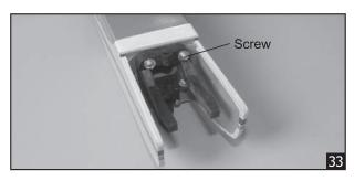
2. Locate the long piece of wire used for the throttle pushrod. One end of the wire has been pre-bend in to a "Z" bend at the factory. This "Z" bend should be inserted into the throttle arm of the engine when the engine is fitted onto the engine mount. Fit the engine to the engine mount using the screws provided.
