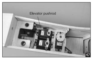
13. Using thick CA glue, secure the pushrod sleeves to the pushrod sleeve guide.
