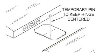
2. Apply six drops of thin CA to the top and bottom of each hinge. Do not use CA accelerator. After the CA has fully hardened, test the hinges by pulling on the aileron.
