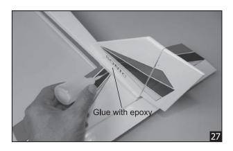
6. Installing the rudder using C.A glue as installing the aileron.
