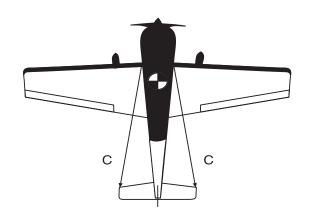
5. Remove the stabilizer. Using the lines you just drew as a guide, carefully remove the covering from between them using a modeling knife.
