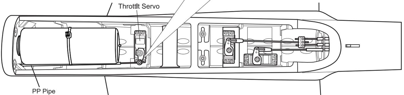
Ensure smooth, non-binding movement when assembling
