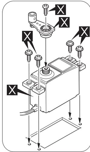
**A** Adjust the throttle input (transmitter throttle stick), throttle trim movement and the carburetor opening to the suitable position and screw in the 4x4mm set screw.
