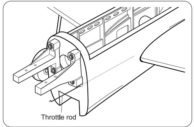
► Temporarily install the engine and make a hole for the throttle rod by aligning with the position of the throttle lever.
