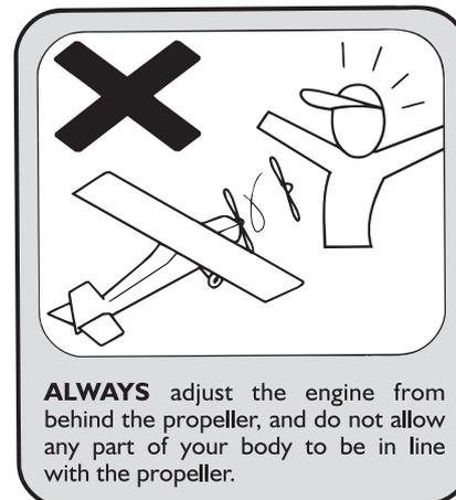
**ALWAYS** adjust the engine from behind the propeller, and do not allow any part of your body to be in line with the propeller.
