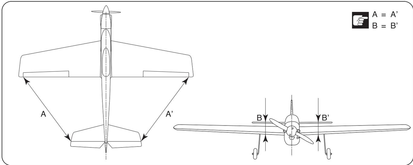
**INSTALLING RUDDER AND TAIL GEAR**
