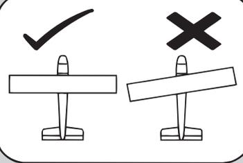
Check that the wings are correctly fitted to the fuselage.
