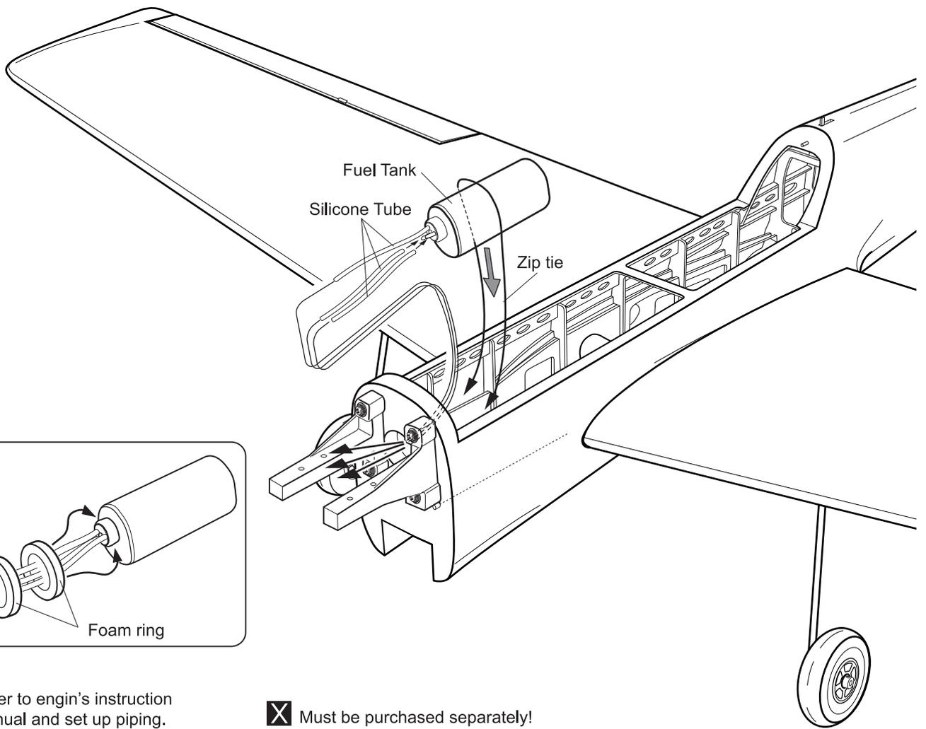
Refer to engine's instruction manual and set up piping.
