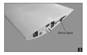
5. Place the aileron servo tray / hatch into the servo box on the bottom of the wing and drill 1,6mm pilot holes through the tray and the servo box for each of the four mounting screws. Secure the servo tray in place using the mounting screws provided (2mm x 12mm).
