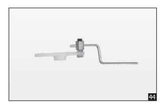
3. Place the servo arm to the servo and secure it.
