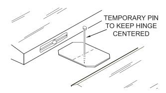
2. Apply six drops of thin CA to the top and bottom of each hinge. Do not use CA accelerator. After the CA has fully hardened, test the hinges by pulling on the aileron.
