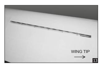
2. Install the air brake into the bay.
