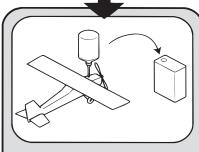
Empty the fuel tank after flying, fuel left in the tank can cause corrosion and lead to engine problems.
