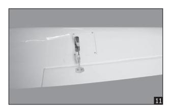
9. Repeat step # 4 - # 8 to install the second aileron linkage. After both linkages are completed, connect both of the aileron servo leads using a Y-harness you have purchased separately.
