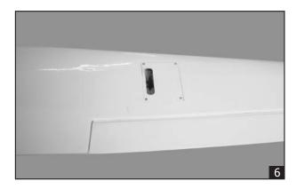
6. Repeat step # 2 - # 5 to install the second aileron servo in the opposite wing half.
