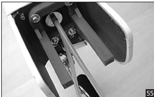
Install the silicon tubes.
