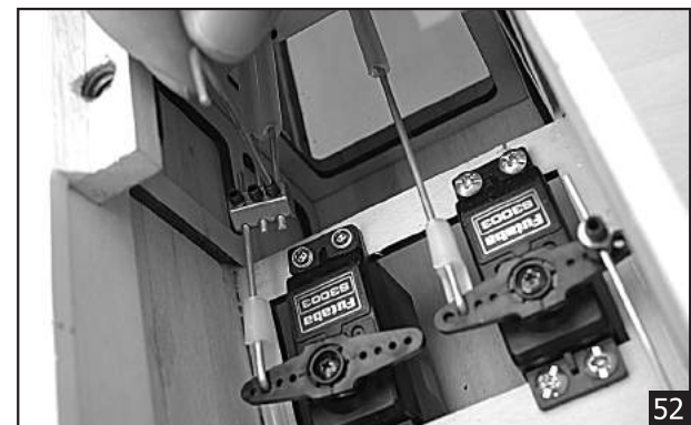
Install the elevator pushrod and secure it.
