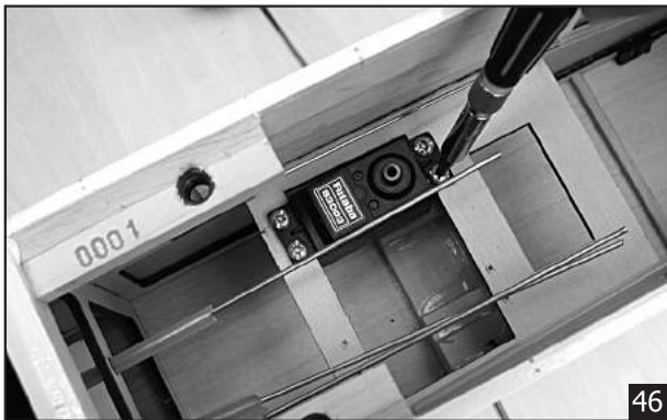
Install the rudder servo.
