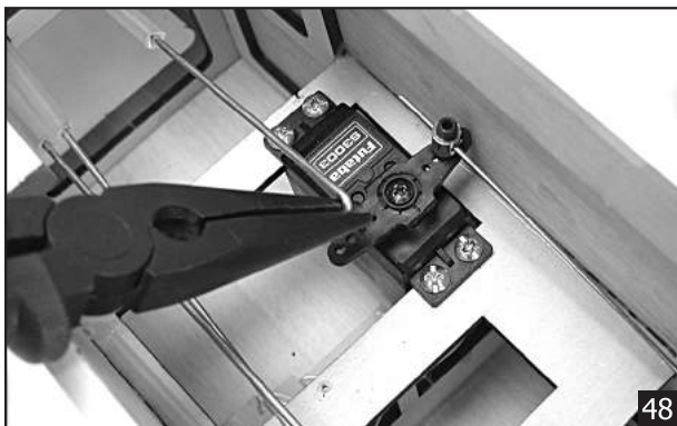
Cut and bend "L" the rudder pushrod.
